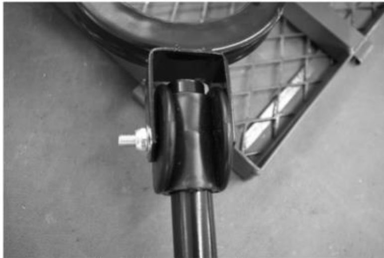
Figure 4: Mounting the handle
