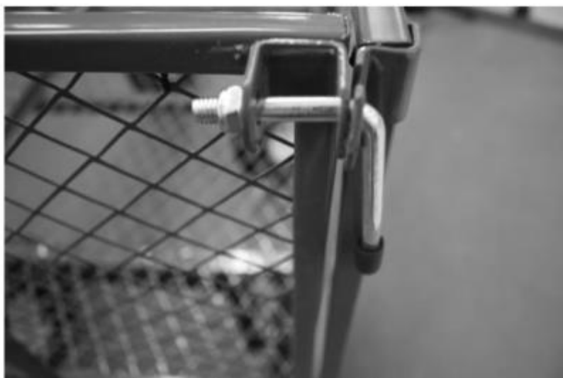
Figure 6: Mounting the "L-bolt"
